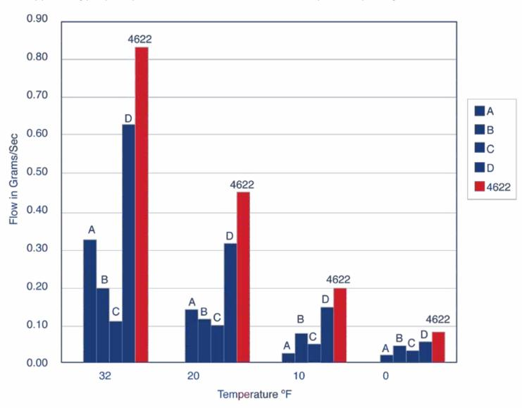
The sample is placed in the pressure cylinder and cold soaked to the prescribed temperature. The flow of grease is started under the selected pressure (usually 150 psi). After the initial flow, sufficient grease is collected to calculate the flow rate in grams of grease per second during a measured amount of time. The higher the flow rate in grams per second, the better the predicted pumpability of the grease.
